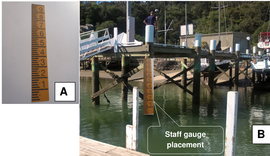
Figure 5. Staff gauge design (photo A) and suggested placement of a staff gauge on wharf pile (photo B).
